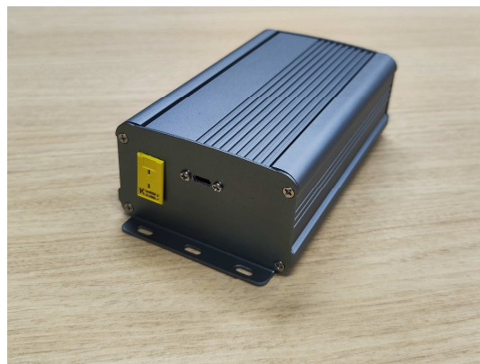
K-type thermocouple terminal and USB B connector
